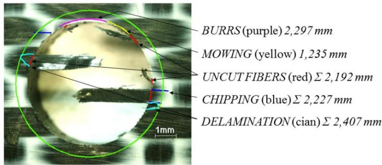
Figure 2. An example of Global Damage measurement.
