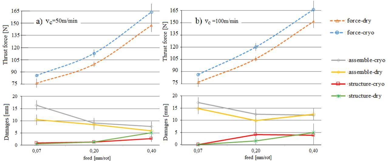
**Figure 4. Damages Vs Thrust force a) at  $v_c=50\text{m/min}$  and b) at  $v_c=100\text{m/min}$**
